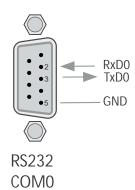
The serial port COM0 is accessible via a 9pin DSUB male connector in the frontpanel of the GPS180, parallel hardwired to the COM0 port on the rear VG edge connector.
